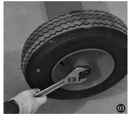
3. Fix the wheel with bearing on the axle of oil tank and fasten the nut with the wrench
