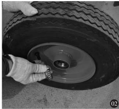
2. Assemble the bearing on each one wheel
