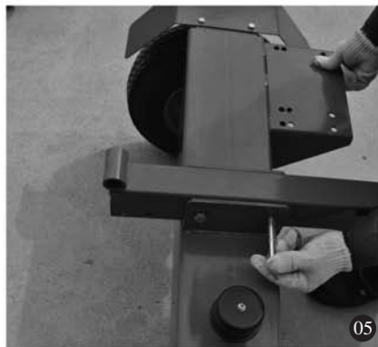
5. Connect the draw pole with the oil tank via bolt and nut
