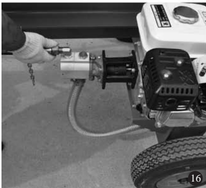
16. Connect the black color oil hose to the oil pump (bend connector of oil pump)
