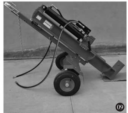
9. Put the bolt back at right position, now the main body is fixed on the draw pole
