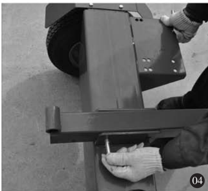
4. Connect the draw pole with the oil tank
