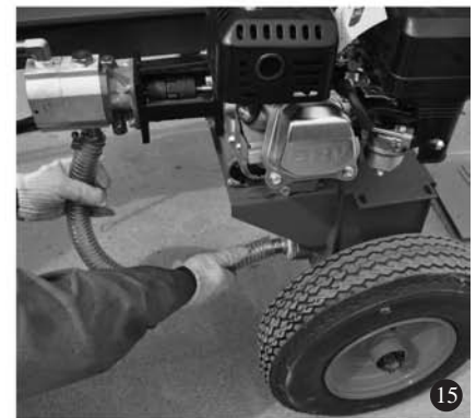
15. Connect the white color oil hose, between the oil pump (undersurface) and oil filter of oil tank and fasten the nut tightly
