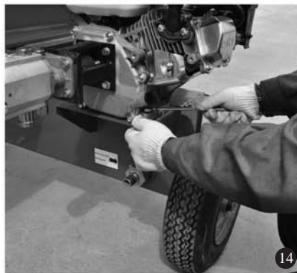
14. Fasten the nut, 4sets of nuts and bolts
