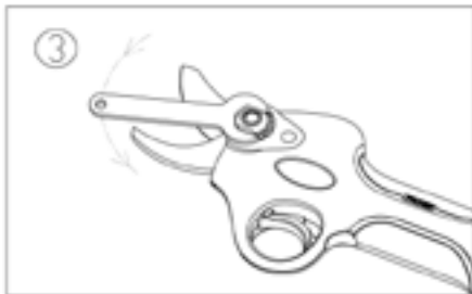
3. Loosen gear nut with crescent wrench.
