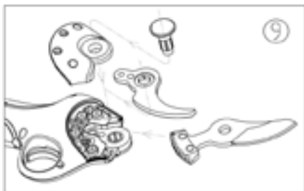
9. Assemble blade set, place cover and insert center bolt.
