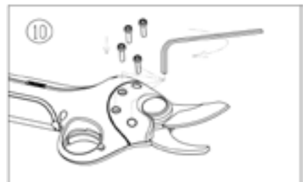
10. Tighten 4 cover screws with allen wrench.
