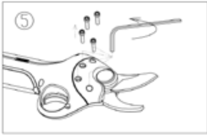
5. Unscrew 4 cover screws with allen wrench.
