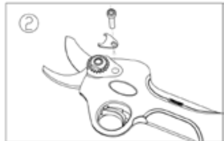
2. Remove adjustment clip bolt and adjustment clip.
