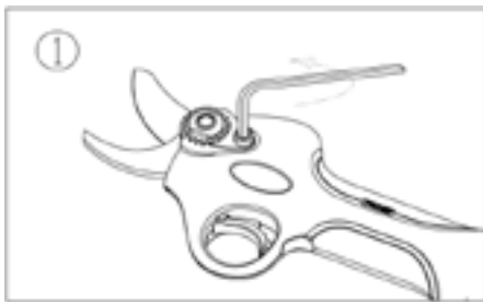
1. Loosen adjustment clip bolt with allen wrench.
