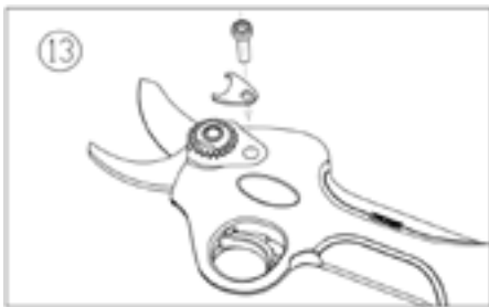
13. Secure gear nut with clip and insert bolt.
