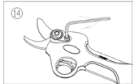
14. Tighten gear nut clip bolt securing the centerbolt gear nut.
