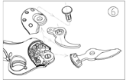
6. Remove cover and disassemble blade set.
