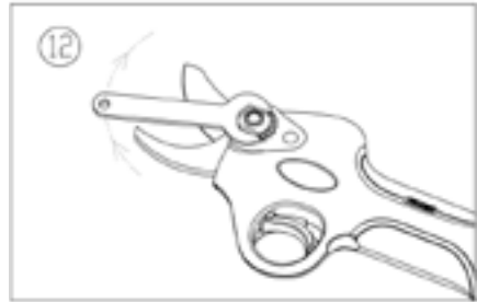
12. Tighten gear nut with crescent wrench.
